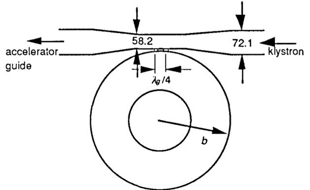
Fig.5 Directional coupler and tapered waveguide.
