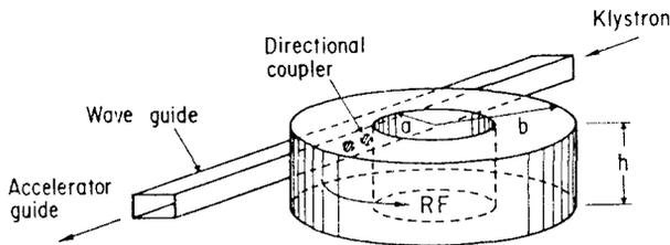
Fig.1 Schematic drawing of a new-type rf pulse compressor using a traveling-wave resonator.
