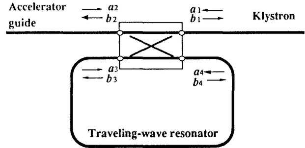
Fig.2 Four-terminal network representation of the pulse-compression system.
