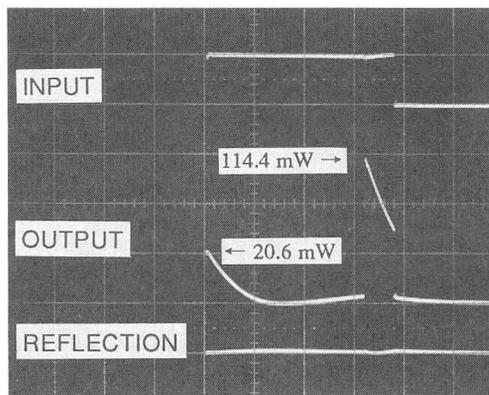
Fig.8 Wave form, input(upper trace), output(center) and reflected.
