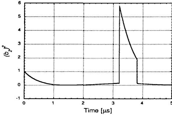
Fig.3 Output wave form from the pulse compressor.
