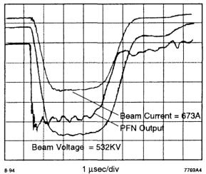
Fig. 2. 400 MW modulator voltage and current waveshapes.
