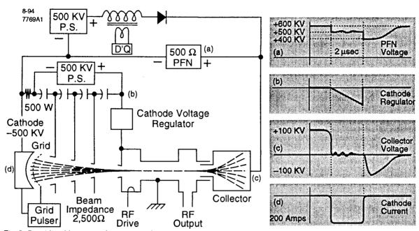
Fig. 3. Quasi-line klystron and power supply system.
