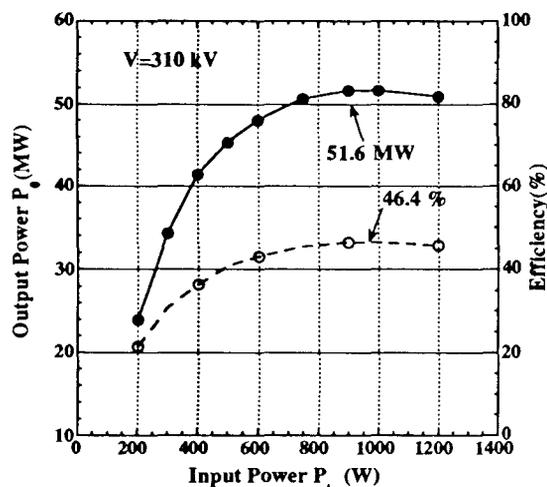
Fig. 3 Input-output power characteristics predicted by the FCI simulation code.
