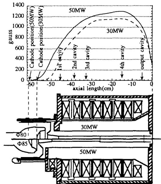
Fig. 1 Relation between the magnet and the tube.
