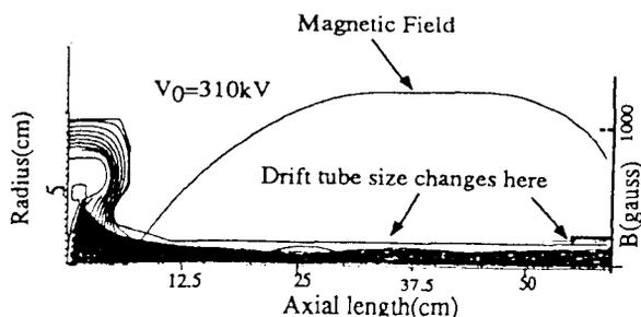
Fig. 2 Beam trajectory at  $V_0=310$  kV.
