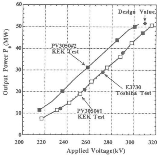
Fig. 4 Test results of prototype 50-MW klystrons.
