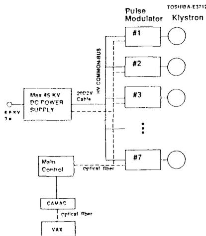
Figure 1. Pulse modulator system with HV common-bus.
