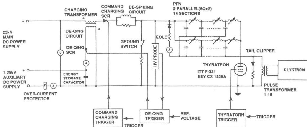
Figure 2. Simplified circuit diagram of the pulse modulator.
