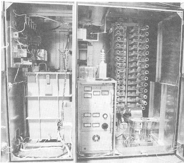
Figure 3. Front view of the pulse modulator.
