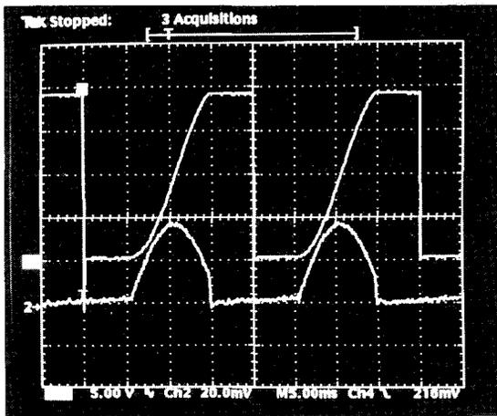
Figure 4. Charging waveforms of PFN.
