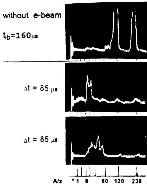
Fig. 4: The time-of-flight spectra of the U high charged ions. Scanning step is  $10\mu s$ ;  $\Delta t = t_{ib} - t_{eb}$
