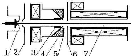
Fig. 1: Schematic of the source design. 1. Electron gun; 2. Collimator; 3. Cathode of MEVVA; 4. Insulator; 5. Trigger; 6. Anode of MEVVA; 7. Drift channel.
