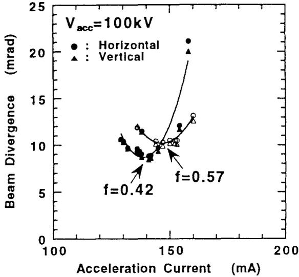
Fig. 2 Beam divergence vs. acceleration current for two field intensity ratio  $f$  of the beam extractor
