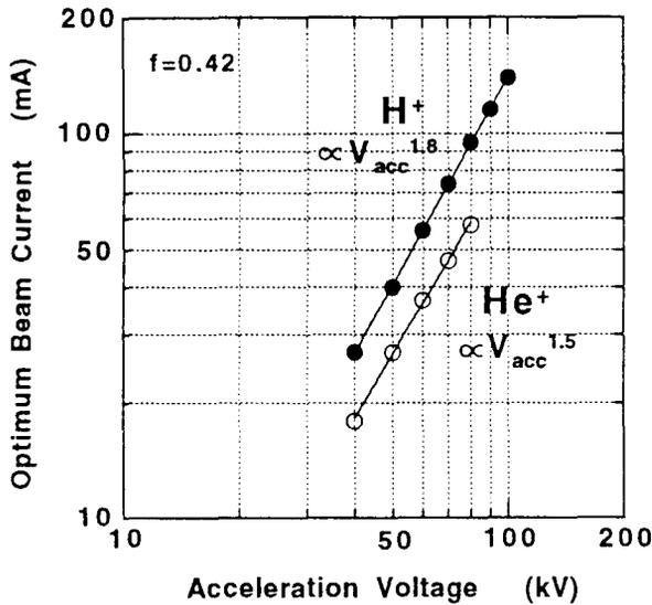
Fig. 5 Optimum current of hydrogen and helium beams
