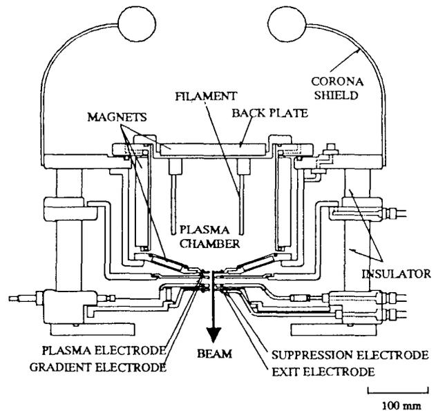
Fig. 1 Cross-sectional view of the ion source
