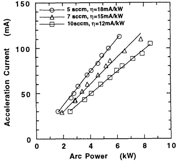
Fig. 3 Arc efficiency for different gas flow rate
