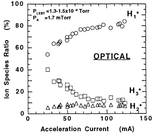
Fig. 6 Ion species ratio vs. acceleration current
