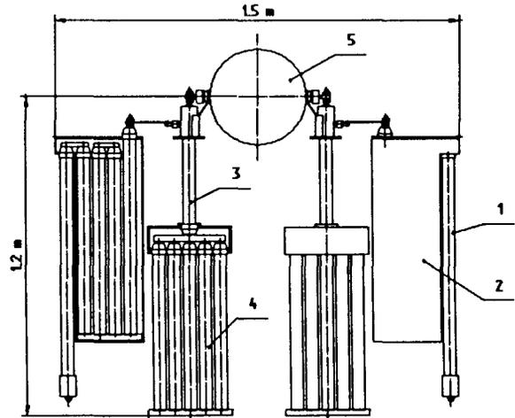
Fig. 5: The design of the SILUND-10 accelerator module, (1) - storage capacitor (*C* in Fig.4), (2) - block of reactors (*L* in Fig.4), (3) - DFL, (4) - NPFL, (5) - induction block.
