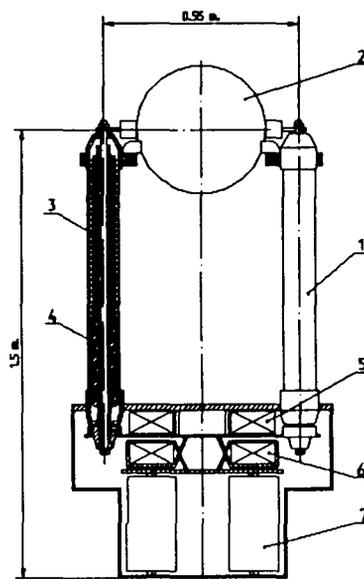
Fig. 3: The SILUND-20 modulator design. (1) - DFL, (2) - induction section, (3) - ferrite rings, (4) - correcting capacity, (5) and (6) - reactors (*L3* and *L2* in Fig.2), (7) - capacitor bank (*C2* in Fig.2).
