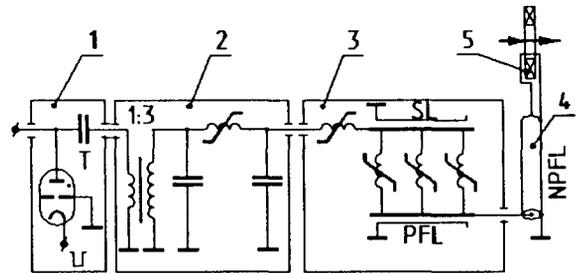
Fig. 6: Scheme the LUEK-20 modulator.
