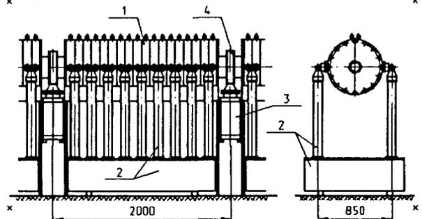
Fig. 1: Accelerating module
