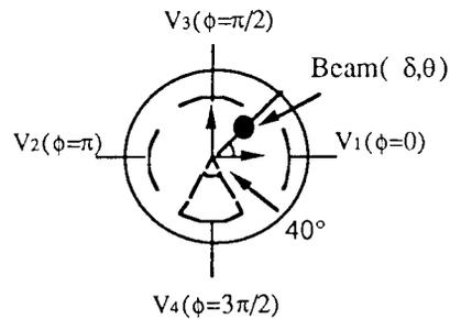
Fig. 2 BPM cross section
