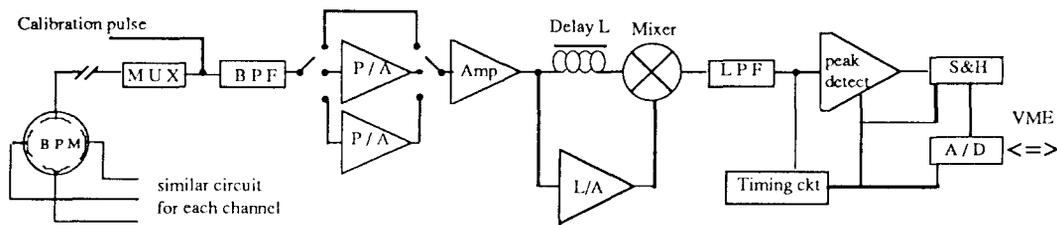
Fig. 1 BPM circuit block diagram.
