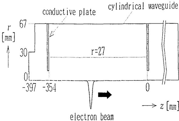
Fig. 1 Analytical model of a symmetric cylindrical waveguide.
