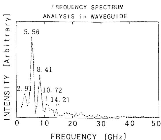
Fig. 4 Frequency spectrum of the spatial distribution on  $r = 27mm$ .
