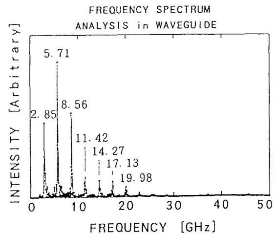
Fig. 3 Frequency spectrum of the temporal distribution for the field component  $E_r(27, -79)$ .
