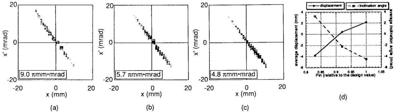
Fig. 3 Dependence of emittance on RF power fed to the DTL,  $P_{in}$
