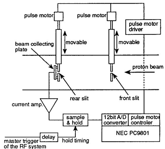
Fig. 1 A schematic diagram of the emittance monitor
