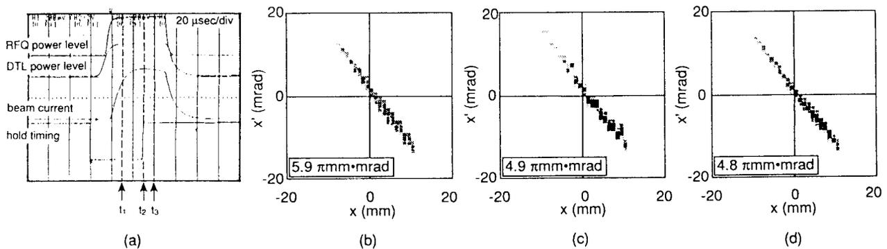
Fig. 4 Dependence of emittance on hold timing,  $t_h$
