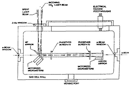
Figure 3: Inverse Cerenkov acceleration gas cell.
