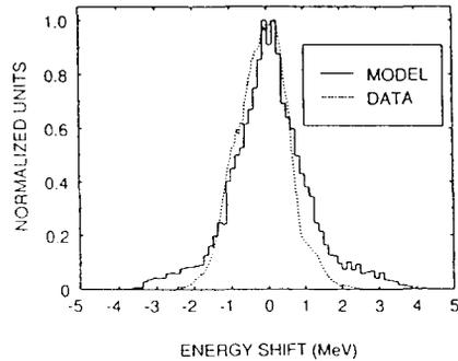
Figure 4: Electron energy spectrum for 0.7 GW laser power.
