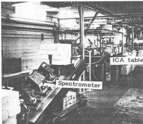
Figure 2: Inverse Cerenkov acceleration beam line.
