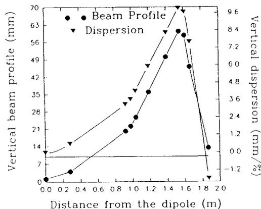
Figure 5: Vertical electron beam profile and dispersion in the spectrometer.
