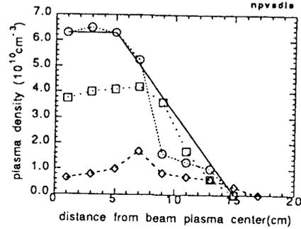
Figure 2: Plasma density distributions along the beam axis. The solid line shows trapezoidal approximation.
