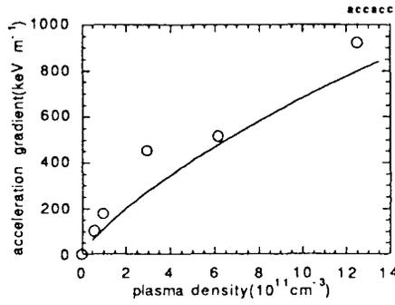
Figure 3: Dependence of acceleration gradient on plasma density. Solid line shows prediction of a linear theory.
