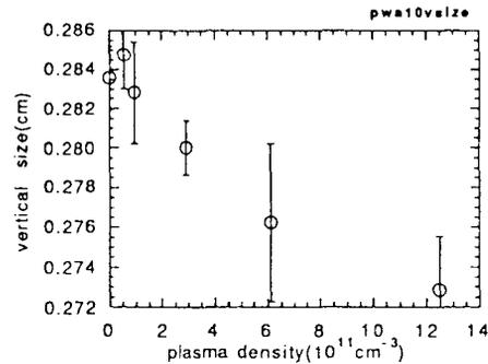
Figure 4: Change caused in energy(a) horizontal beam width(b) and vertical width(c) of the drive bunches as functions of plasma density.
