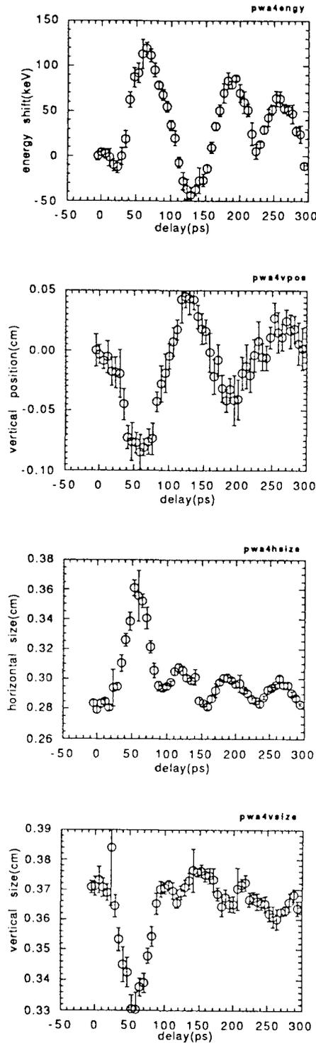
Figure 1: Each example of time dependence of (a)energy change, (b)vertical position, (c)horizontal beam size, and (d)vertical beam size of test bunches. Plasma density was  $6.14 \times 10^{11} \text{cm}^{-3}$ .
