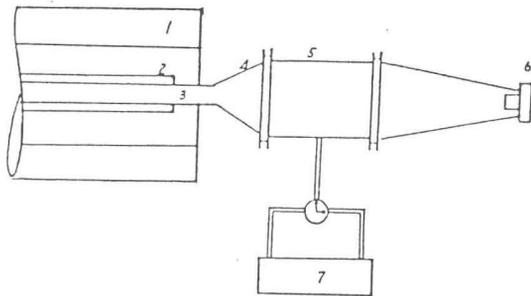
Fig. 2. Schematic diagram of experimental system for observing operating mode in a Raman free electron laser. 1, guide magnet, 2, wiggler magnet, 3, drift tube, 4, output horn, 5, low pressure gas chamber, 6, camera, 7, pumping and filling gas system.
