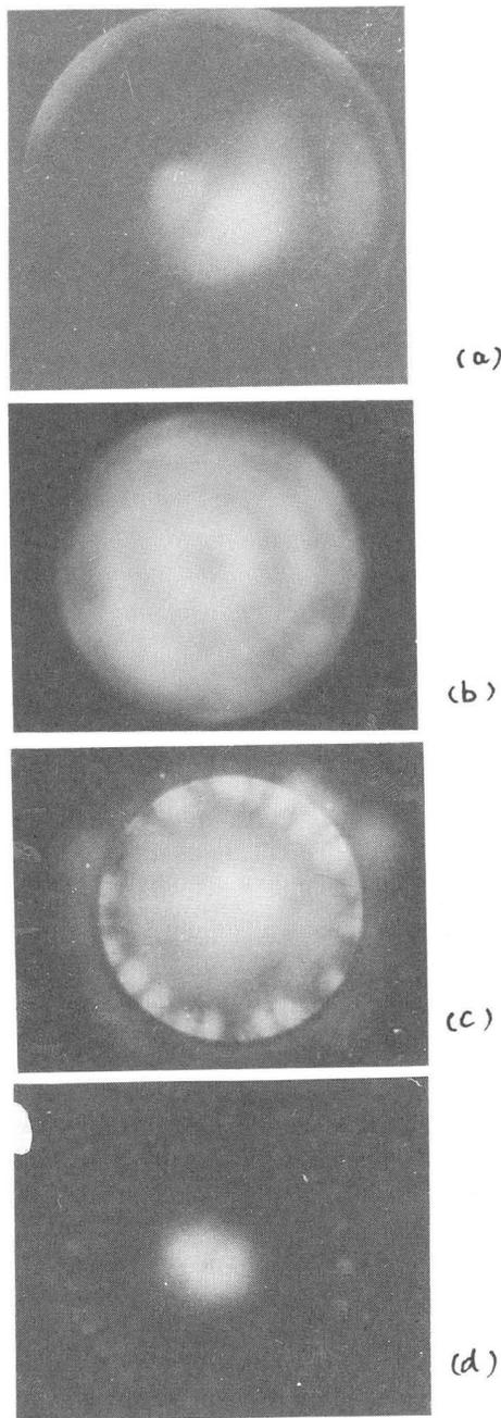
Fig.4. Photographs of microwave-induced gas breakdown for illustrating the mode observation,  $B_0=7150$  G,  $\beta_{\perp}=0.58$ .
