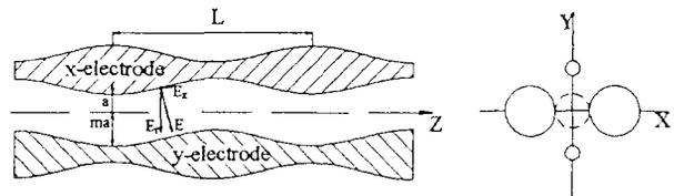
Fig. 2 Scheme of the modulated RFQ electrodes
