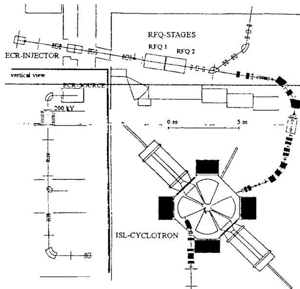
Fig. 4 Layout of the Cyclotron with the new Injector
