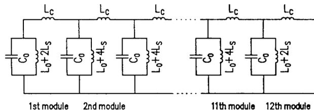
Figure 2: Equivalent circuit of the 12-module cavity.
