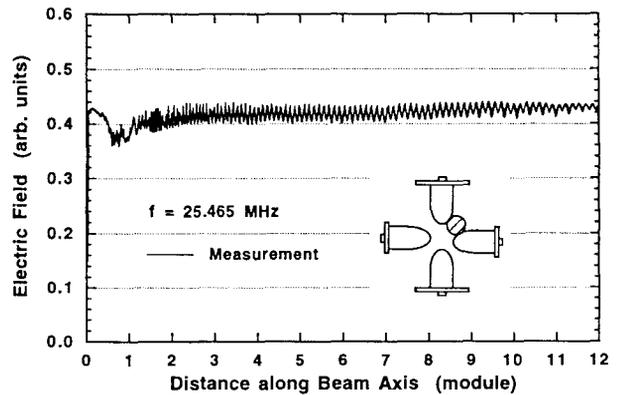
Figure 5: Azimuthal field balance after tuning. Four curves for the quadrants are plotted
