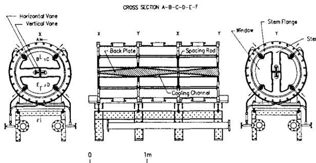
Figure 1: Structure of the unit cavity.
