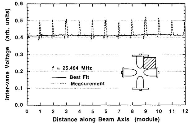
Figure 4: Longitudinal voltage distribution after tuning.
