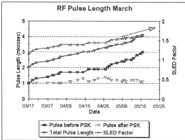
Fig. 5: RF pulse width during the commissioning
