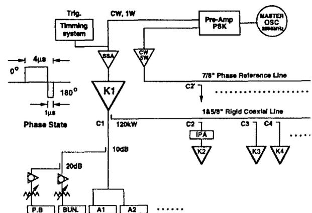
Fig. 2: Schematic diagram for RF drive system
