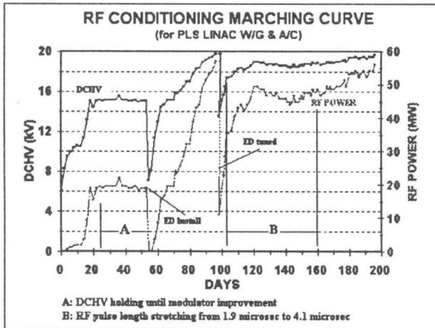
Fig. 3: Typical RF conditioning for new module
