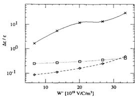
Fig. 1 Emittance dilution versus wakefield strength for 3 cases: (solid) no correction, (dashes) correction varying charge and bunch length, and (dots) correction varying only charge; in the SLAC NLC design,  $W' = 7 \times 10^{19} \text{ V/C/m}^3$ .
