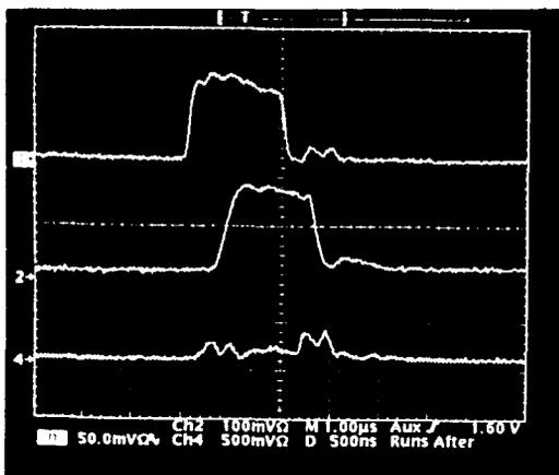
Fig. 5 RF pulse waveforms of input (upper), output (middle) and input reflection (lower).
