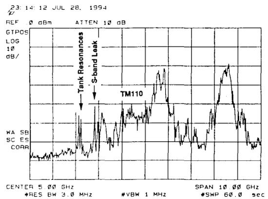
Fig. 6 Wake field spectrum. Theoretically expected (upper) and measured (lower) spectrum.
