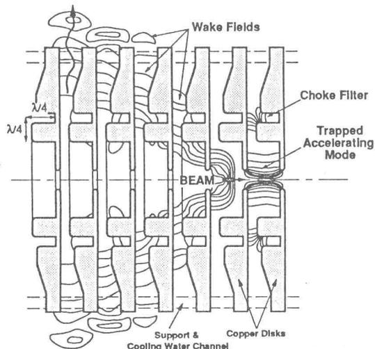
Fig. 1 Concept of the HOM-free choke-mode accelerating structure.
