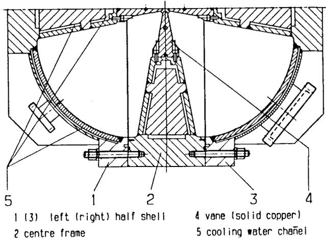
Figure 6: Conceptual design study - lower half cross section of the proposed 4 vane RFQ.
