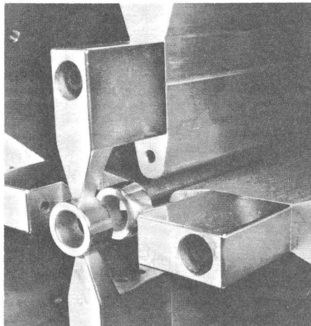
Figure 1: Separation of dipole modes by shorting together vane pairs at the high energy end with a drift tube.
