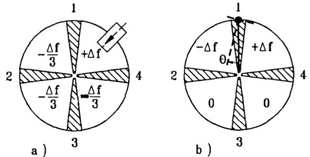
Figure 3: Comparison of two detuning mechanisms: (a) Detuning of one quadrant by a pair of cylindrical plungers; (b) Detuning of two quadrants by the displacement of one vane by an angle  $\Theta$ .
