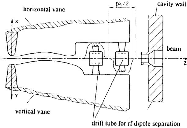
Figure 2: Sketch of the geometry at the high energy end of the modulated vanes.
