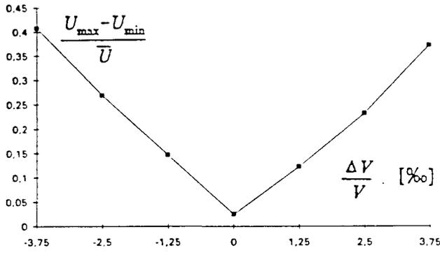
Figure 4: Effect of the relative volume change  $\Delta V/V$  inside one quadrant on the maximum relative deviation of the four vane-vane potentials, without drift tubes; volume changed by plungers.
