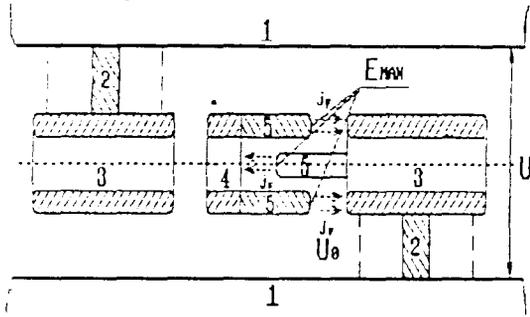
Figure 1. Accelerating period of the SPRFQF structure. 1 - H-cavity; 2 - electrodes holders; 3 - electrodes; 4 - intermediate electrode; 5 - focusing "horns".
