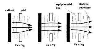
Fig. 1 The diagram of electron trajectory near a single aperture grid. The trajectory differs with electric field(shape of equipotential line) near the grid. Va : voltage between anode and cathode. Vg : voltage between grid and cathode.
