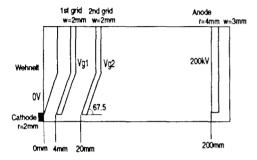
Fig.2 The geometry of the electron gun with double grids.
