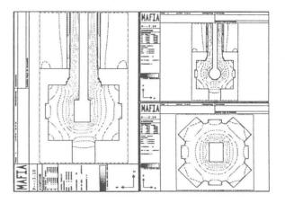
**Fig.6** Equipotential contour plot of MAFIA results. Left : a cross section cutting by y-z plate. Upper right : a cross section cutting by x-y plate. Lower right : a cross section cutting by x-z plate.
