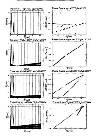
Fig.4 Plots of EGUN results for each conditions. Left : Beam Trajectories. Right : Phase Space Plots.
