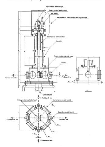
**Fig.5** The design scheme of a new gun system to be possible to measure the gun performance including cathode condition with installing in beam line of the linac.
