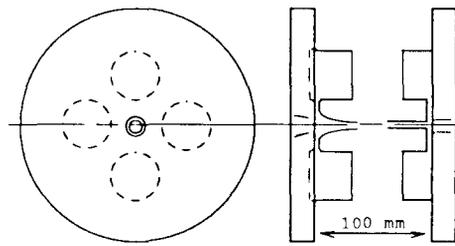
Fig. 5 A schematic drawing of the end plate at the entrance and the both vane end regions.
