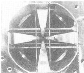
Fig. 1 A photograph of the PISLs installed to the JHP RFQ.
