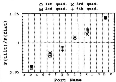
Fig. 8 Distribution of the squares of magnetic field strengths in the four quadrants measured with the loop monitors after inserting two movable tuners at a\_ports by 5 mm and extracted two movable tuners at o\_ports by 5mm.
