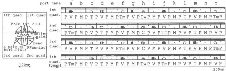
Fig. 2 A cross-sectional view of the RFQ cavity and longitudinal views of the four quadrants of the cavity. The characters of P, C, T, Tw, Tm, V and M stand for PISL, coupler, stab-tuner, stab-tuner with viewing hole, movable tuner, vacuum port and loop monitor, respectively.
