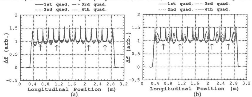
Fig. 4 Distribution of the squares of magnetic field strengths in the four quadrants measured with bead perturbation method : (a) before tuning and (b) after tuning.
