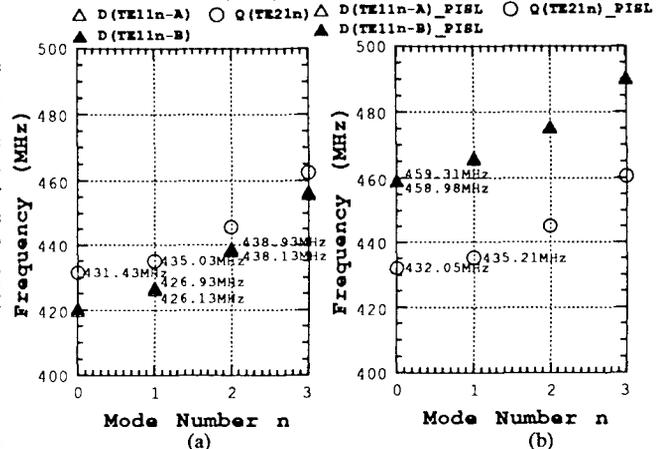
Fig. 7 Measured dispersion curves: (a) in the cold model without PISLs and (b) in the JHP RFQ.
