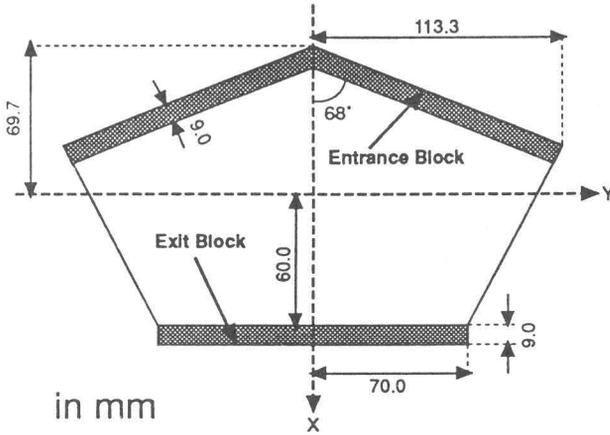
Fig. 3: The shape of the iron pole of the new Mixing Magnet.
