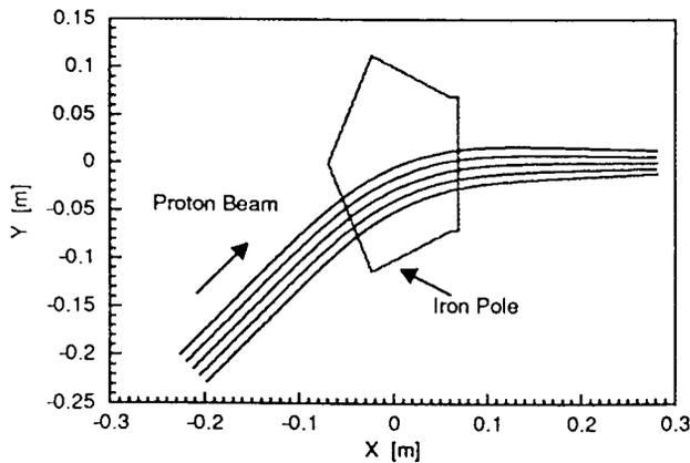
Fig. 7: The several orbits on the median plane. The distance between the neighboring orbits is 1 cm before entering Mixing Magnet.
