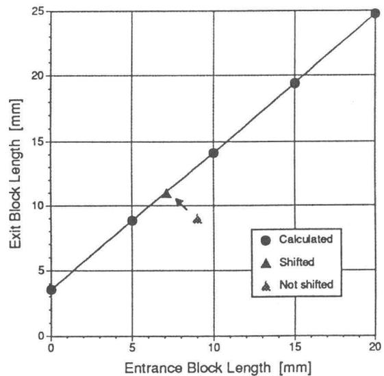
Fig. 5: The relation between the length of the entrance block and that of the exit block.
