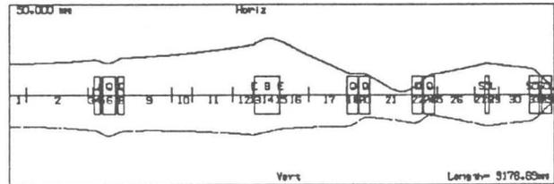
Fig. 2: Beam envelopes calculated by TRACE-3D at a current of 20 mA.
