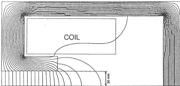
Fig. 4: The 2-dimensional field calculation by POISSON.
