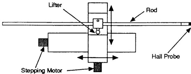
Fig. 6: The schematic view of the field measurement system.
