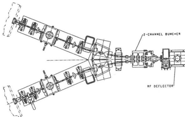
Fig. 1. This plot shows the front-end part of the APDF. The beams from the two ion-sources are deflected into a common channel. The two cavities of the final step of the deflection will be discussed here.
