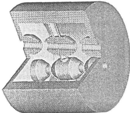
Fig. 4. This is a structural model of the two beam buncher cavity. The strong bunching is achieved by using two gaps within a single cavity.
