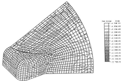
Fig. 3. The Von Mises stresses for the heat loads calculated with MAFIA and the provided cooling.
