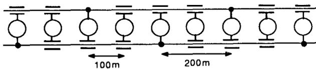
Fig.5 Stretched-wire alignment chain for CLIC
