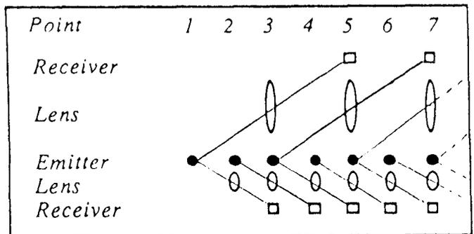
A statistical analysis of this redundant set of measurements enables the absolute displacements of the articulated points in space with respect to the ideal straight line to be determined and the necessary movements of the jacks to be calculated to minimise the excursions. Such a system would necessarily be connected to a computer so that the
