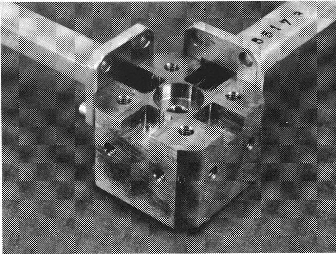
Fig. 6 CLIC prototype beam position monitor
