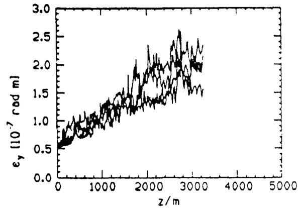
Fig.11 Vertical emittance blow-up along the CLIC linac for the one-to-one correction scheme (500 GeV c.m.)
