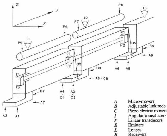
Fig.2 Support, movement and measurement system
