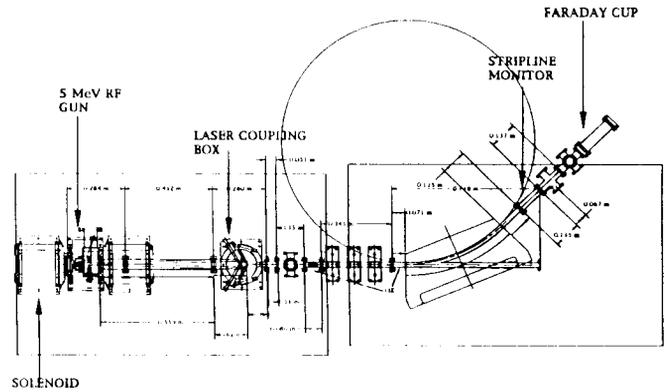
Figure 1: Experimental setup. There are same diagnostics for straight beams too, but not shown here for simplicity.
