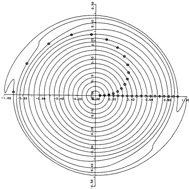
Fig. 1 Solutions of equ. (1) in phase space after 4 betatron oscillations for  $I/I_{\max} = 0.44$ . Particle states \* correspond to initial states  $\hat{v}$ , resp.
