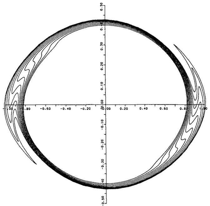
Fig. 2 Behaviour of outer particles for  $I/I_{\max} = 0.47$  in phase space after 4 betatron oscillations
