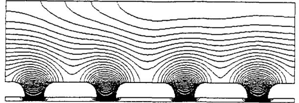
Figure 1: Field lines obtained by running SUPERFISH for the first four cells in Tank 3 before modifications were made.
