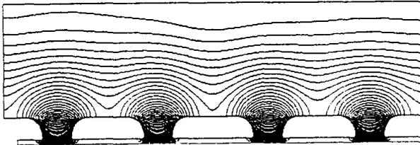
Figure 2: Field lines obtained by running SUPERFISH for the first four cells in Tank 3 after modifications were made.
