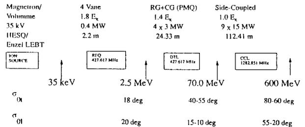
Figure 1: SSC linac block diagram.
