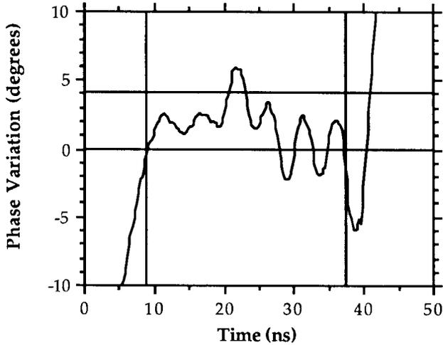
Figure 1. Phase variation of the rf output pulse.
