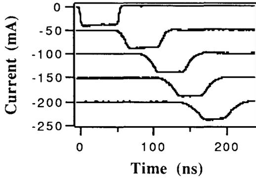
Fig. 5. Beam waveforms for drift expansion.
