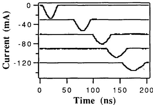
Fig. 2. Beam current waveforms for drift expansion.
