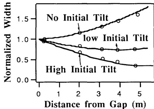
Fig. 4. Normalized bunch width vs. drift distance for parabolic bunches where the solid curves represent theory and the circles experiment.
