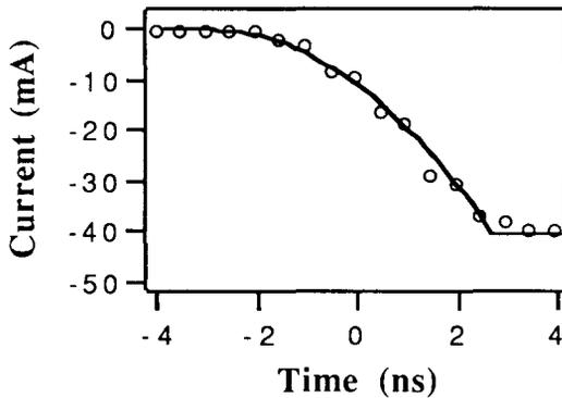
Fig. 7. Leading edge of first waveform in Fig. 5. the solid curve represents theory and the circles experiment.
