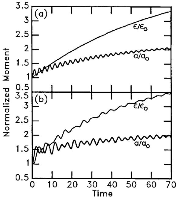
Fig. 1. RMS beam size and emittance, normalized to  $t=0$ , (a) from harmonic-oscillator model of particle orbits with  $(\omega_n/\omega_0)^2 = 1.5$  and  $\beta = 0.015$  in the limit  $\beta_s \rightarrow \infty$ ; (b) calculated self-consistently with  $(\omega/\omega_0)^2 = 1.5$ ,  $(\omega_p/\omega_0)^2 = 1.4$ ,  $\beta_s/\omega_0 = 1.0$ , and  $\beta/\omega_0 = 0.015$ .
