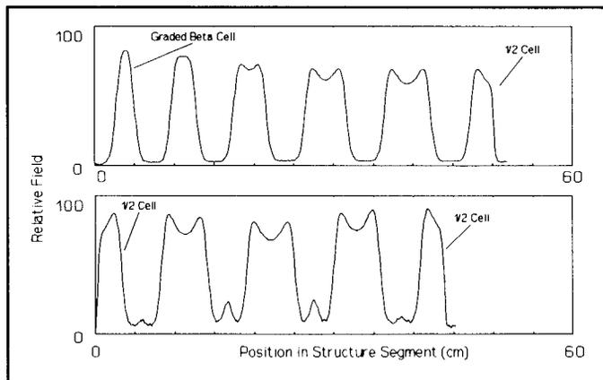
Fig. 2 Graded-beta and coupling sections of linac.
