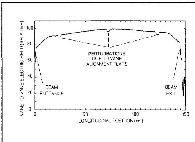
Fig. 5 RFQ longitudinal field distribution.
