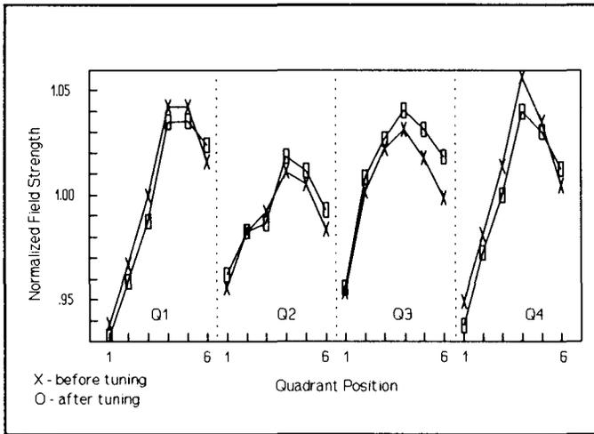
Fig. 4 Azimuthal field measurements in an RFQ.
