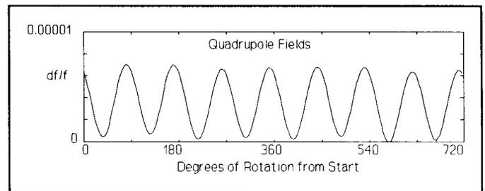
Fig. 3 Quadrupole field measurement.
