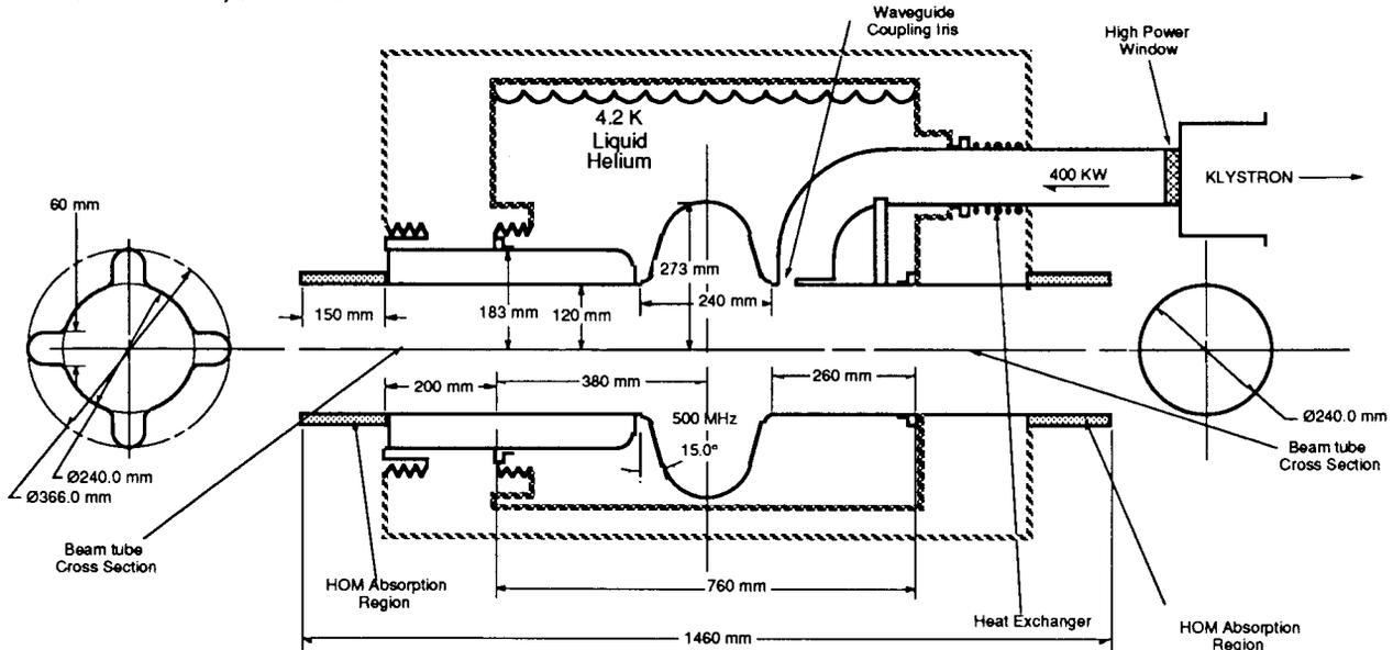
Fig. 3 Proposed Accelerating Cavity System
