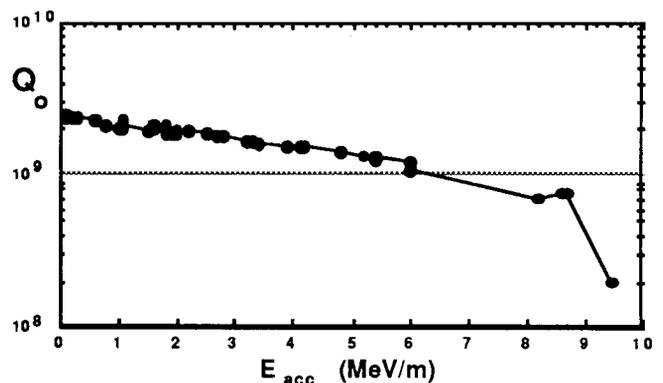
Fig. 4  $Q$  vs.  $E_{acc}$  for B Cell Test
