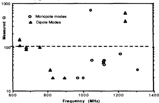
Fig. 5 Q vs. Frequency for Damped Cavity
