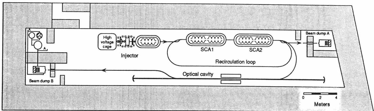
Figure 1. Overall Configuration of Components in Shielding Vault
