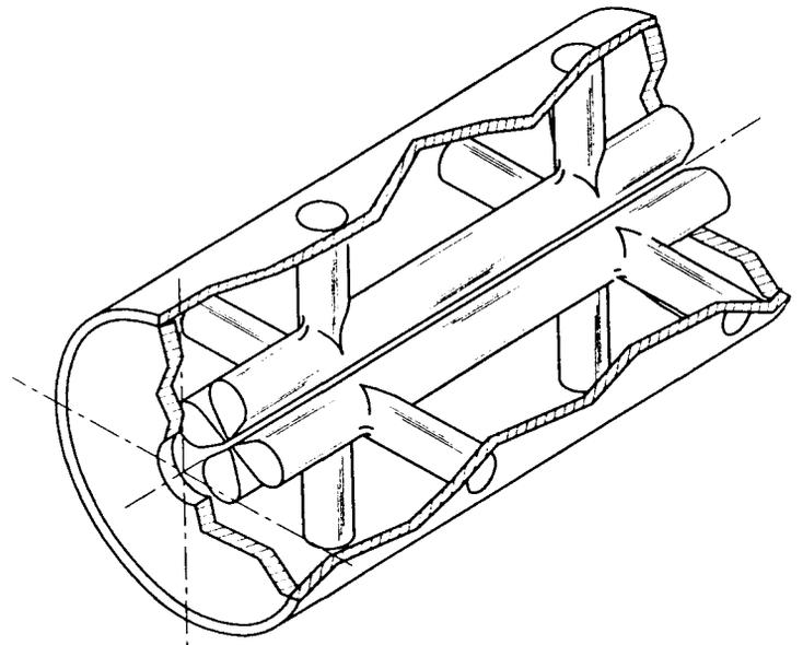
Fig. 1 194 MHz, four-fold symmetric rod and post structure. The vanes or rods are 50 cm long. The relatively large diameter of the rods is not only practical in a superconducting structure, but desirable for good mechanical stability.
