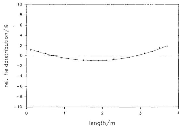
Fig. 7 Field distribution along the RFQ prototype
