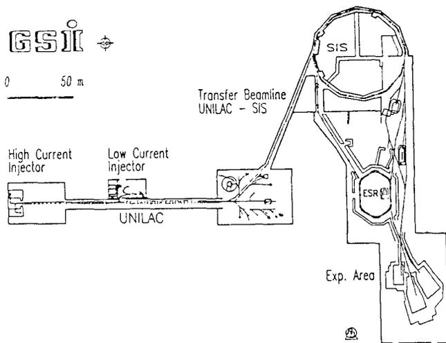
Fig. 1 Plan view of the extended GSI accelerator facilities
