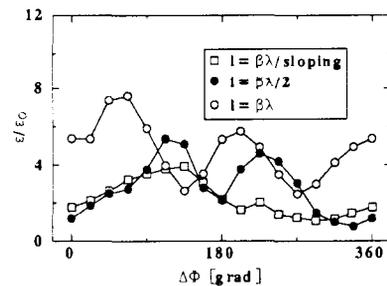
Fig. 5. The emittance growth as a function of the relative rf-phase  $\phi$  at a beam current  $I$  of 0.1 mA. The deflector voltage is the same as in Fig. 4.
