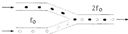
Fig. 1. Principle of a two channel funneling line.
