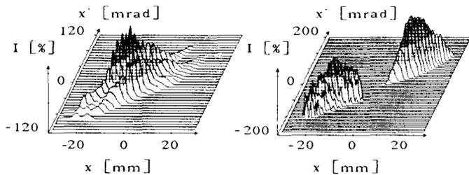
Fig. 7. The 3d  $x, x'$ -emittance at a deflector voltage of 20 kV. On the left:  $\Delta x' = 0$  ( $I = \beta\lambda$ ), on the right:  $\Delta x_{max}$  ( $I = \beta\lambda/sloping$ ). The beam current  $I$  is 1.2 mA.
