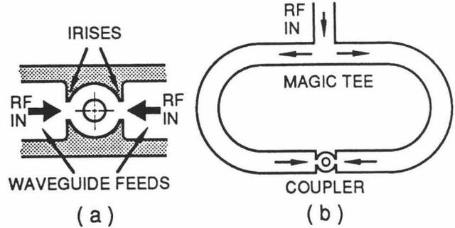
Fig. 1 Schematics of RF power input to coupler.
