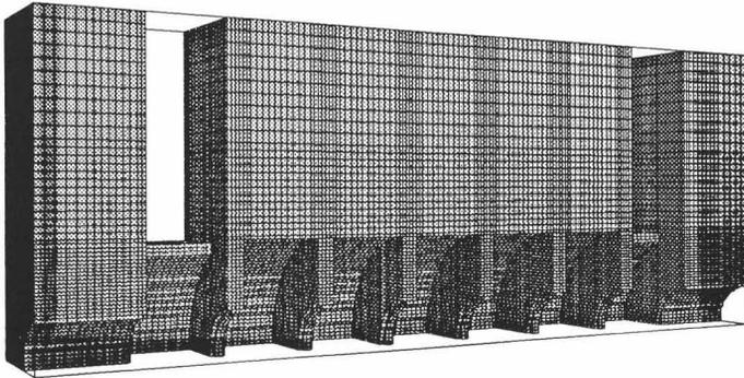
Fig. 4 MAFIA geometry for a 7-cavity traveling wave section.
