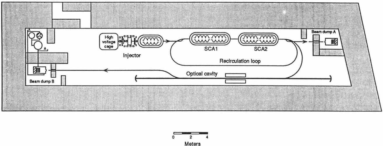
Fig. 1: Layout of IRFEL inside the Vault of the CDRL Building.
