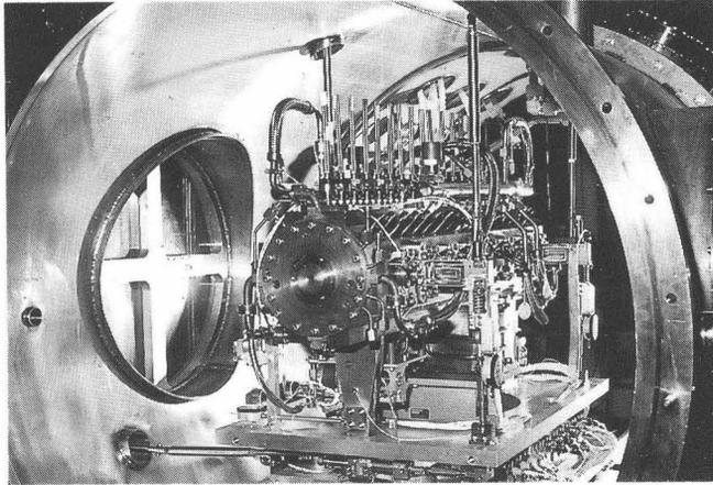
Fig. 2 DTL Module Installed in the LPCTB.
