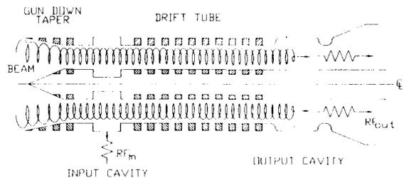
Figure 4. A coaxial second harmonic two-cavity circuit.
