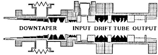
Figure 1. The two-cavity microwave circuit configuration.
