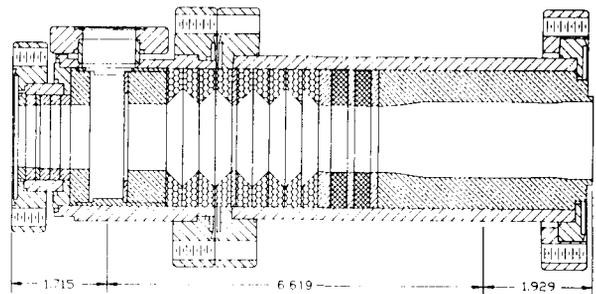
Figure 3. The initial two-cavity second harmonic circuit configuration.
