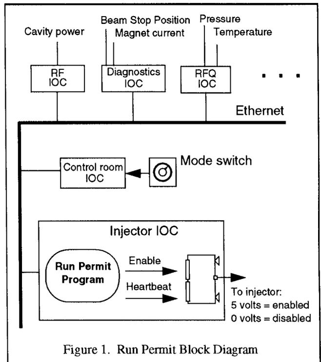
Figure 1. Run Permit Block Diagram
