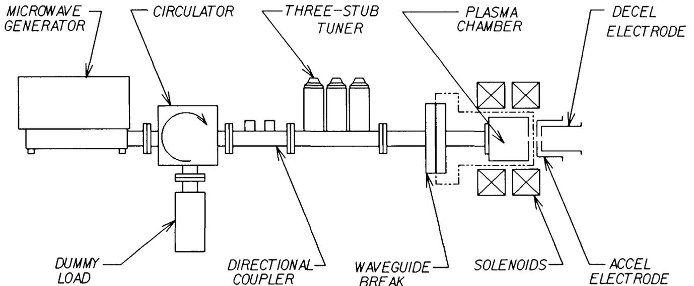
Fig. 1 Chalk River ECR ion source system. Only the components enclosed by the dashed line are at the extraction potential.
