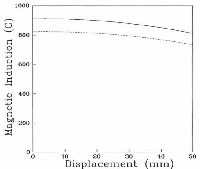
Fig. 3 Magnetic induction on the axis of the ion source as a function of the displacement from the microwave window. The solid and dashed lines correspond, respectively, to on- and off-resonance operation.
