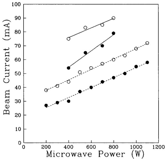
Fig. 4 Total beam current (open symbols) and proton beam current (closed symbols) on-resonance (solid lines) and off-resonance (dashed lines) as a function of microwave power at a hydrogen mass flow of 1.0 sccm (1.5  $\mu\text{g/s}$ ).
