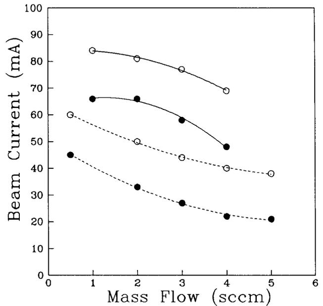
Fig. 5 Total beam current (open symbols) and proton beam current (closed symbols) on-resonance (solid lines) and off-resonance (dashed lines) as a function of hydrogen mass flow at a microwave power of 600 W.
