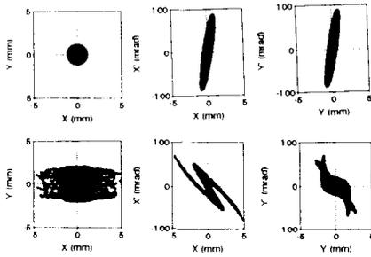
Figure 4: Modified PARMILA results on particle distribution for  $H^-$  beam from the SSCL magnetron source. Top: input to the ESQ LEBT. Bottom: output from the ESQ LEBT.
