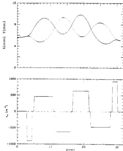
Figure 2: Linear beam optics result for a parallel input beam. Top: Amplitude (X, Y) of the beam envelope through the ESQ LEBT along x (solid line) and y (dotted line); bottom: focusing function,  $\kappa$ .  $z$  is the direction of propagation of the beam.
