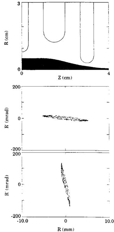
Figure 3: SNOW-2D results for the einzel lens module. Top: Beam trajectory through the einzel lens module. The center electrode is at  $-36$  kV and the two end electrodes are grounded. Middle: Phase-space distribution of the input beam. Bottom: Phase-space distribution of the output beam.
