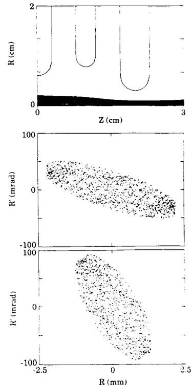
Figure 5: SNOW-2D results for the einzel lens module. Top: Beam trajectory. The center electrode is at  $-36$  kV. Middle: Phase-space distribution of the input beam (Effective values from Fig. 4 are used to model it.) Bottom: Phase-space distribution of the output beam.
