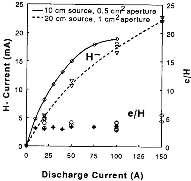
Fig. 2 - Comparison of the H<sup>-</sup> current and electron-to-H<sup>-</sup> ratio vs. discharge current for the 10 cm and 20 cm diameter BNL sources.
