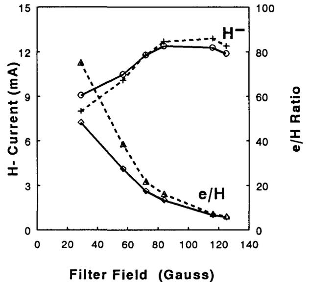
Fig. 4 - H<sup>-</sup> current and electron-to-H<sup>-</sup> ratio as a function of the strength of the conical filter field. Dotted line: plasma electrode floating; solid line: plasma electrode grounded. Discharge current = 50 A.
