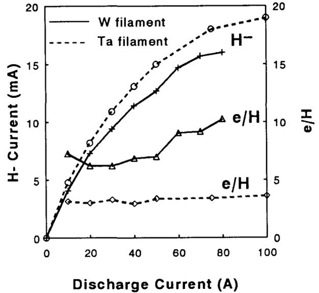
Fig. 3 - H<sup>-</sup> current and electron-to-H<sup>-</sup> ratio vs. discharge current when operating the source with tungsten and tantalum filaments.
