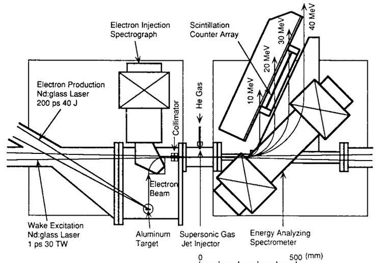
Figure 2: Experimental layout for electron acceleration
