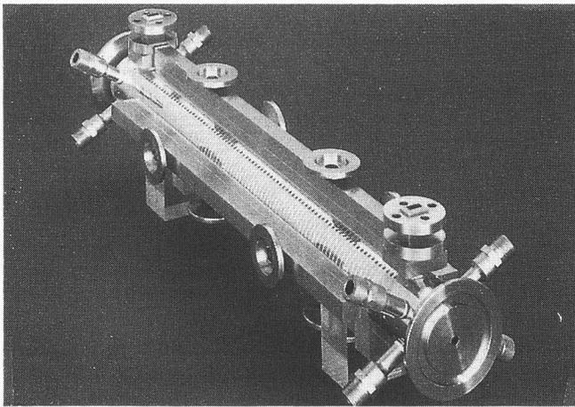
Fig. 2 The 30 GHz prototype CLIC accelerating section
