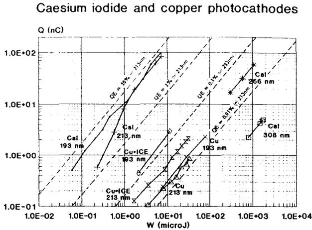
Fig. 4 Charge as function of the laser energy of the photocathode - ICE: Ion Controlled Etching
