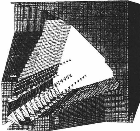
**Fig. 4** Three-dimensional RFQ structure with vane end region generated with MAFIA. Arrow shows the electric field vector.
