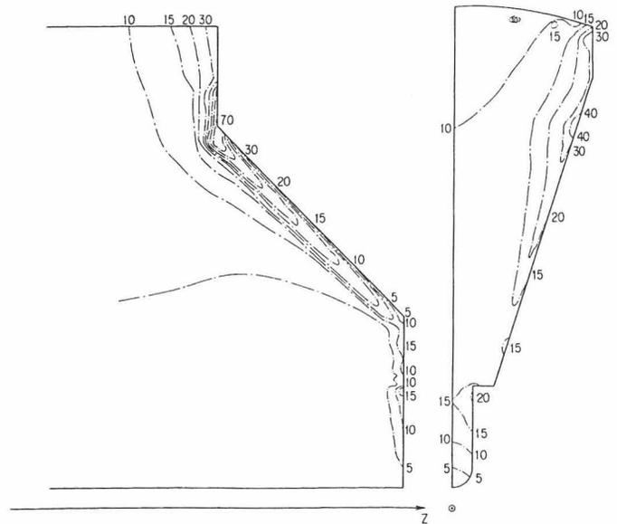
**Fig. 7** RF peak power loss density in  $W/cm^2$  along the surface of the vane. (60%Q is assumed.)
