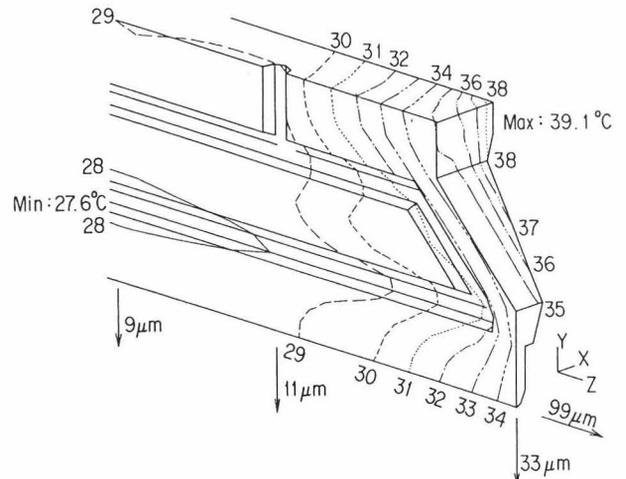
**Fig. 8** Temperature distribution and displacement of the RFQ vane
