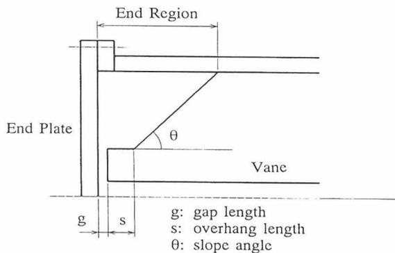
**Fig. 5** Cross section of the RFQ end region
